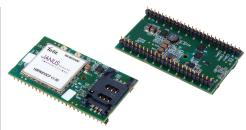
The HSPA910CF v1.00 CF Plug-In modem incorporates Telit's HE910 penta-band module as its cellular heart. The unit operates in the GSM, GPRS, EDGE, UMTS, or HSPA+ bands, defaulting to the appropriate network. It is pin compatible with the full line of Janus Plug-In Terminal products.
