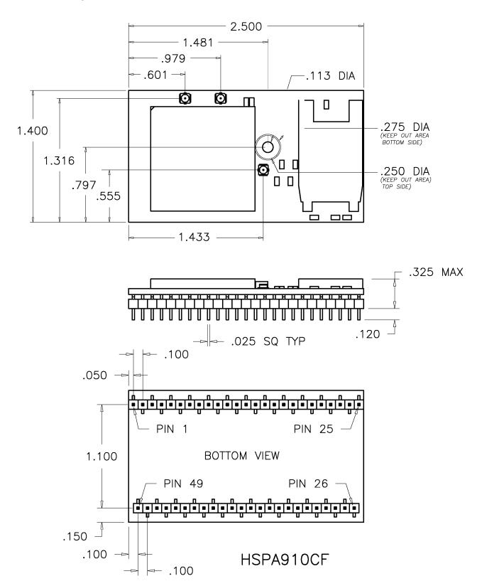
Figure 18 HSPA910CF Mechanical Dimensions
