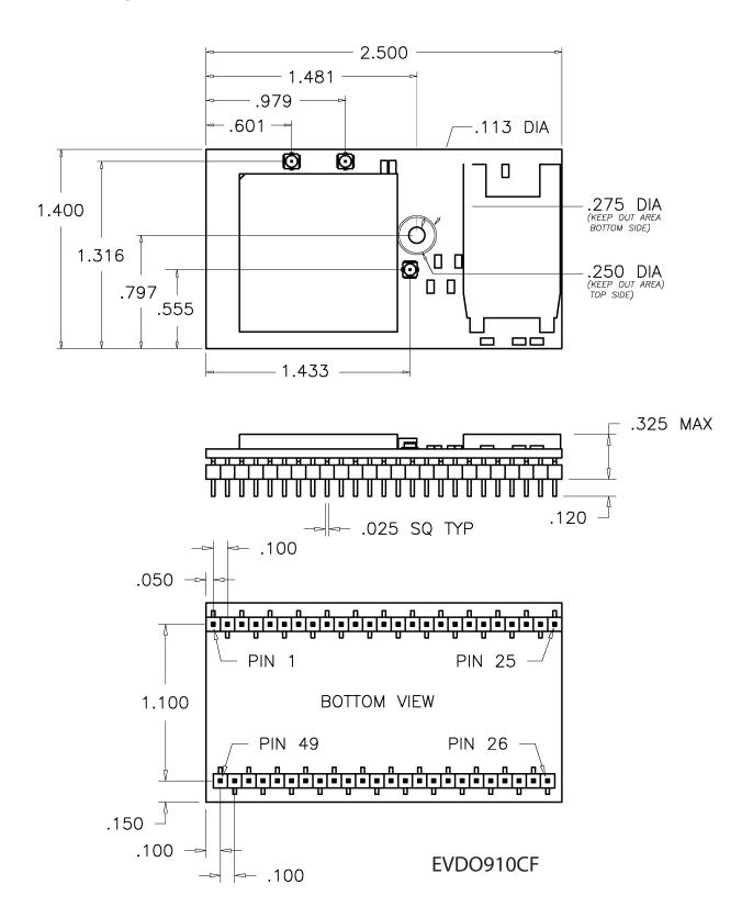
**Figure 18 EVDO910CF Mechanical Dimensions**
