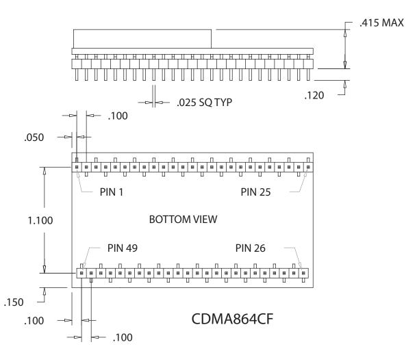
Figure 16 CDMA864CF Mechanical Dimensions
