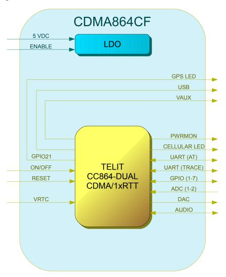
**Figure 2 CDMA Block Diagram**
