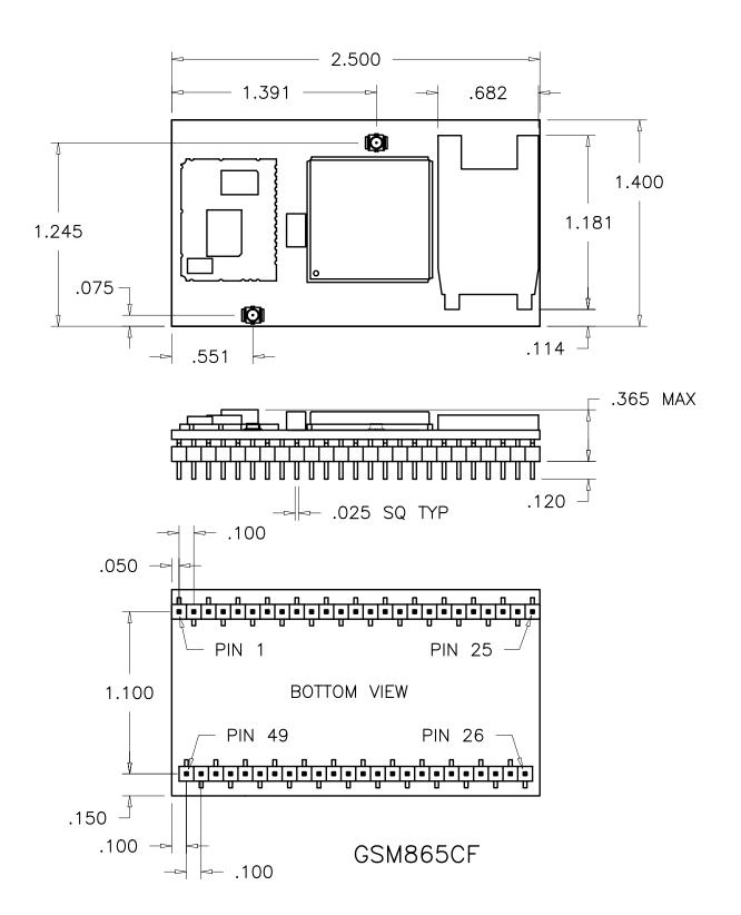
Figure 15 GSM865CF Mechanical Dimensions
