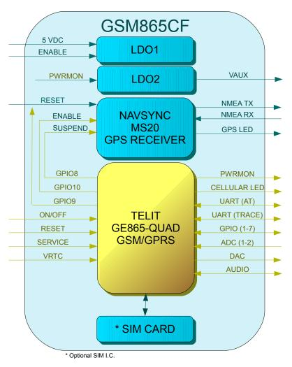
**Figure 1 GSM Block Diagram**
