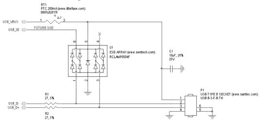
Figure 7 USB Connection Diagram
