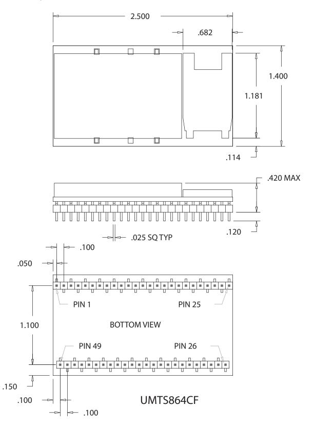
Figure 17 UMTS864CF Mechanical Dimensions
