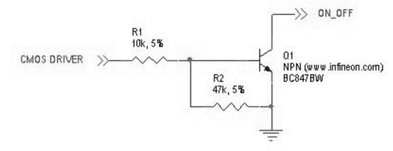
Figure 12 On / Off Pin Diagram
