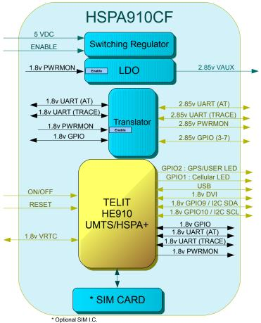
Figure 4 HSPA910CF Block Diagram
