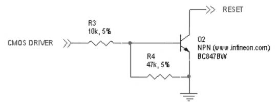
Figure 11 Reset Pin Diagram9
