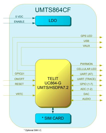
**Figure 3 UMTS Block Diagram**
