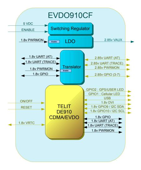
Figure 5 EVD0910CF Block Diagram
