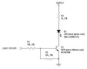
Figure 13 LED Indicators Diagram
