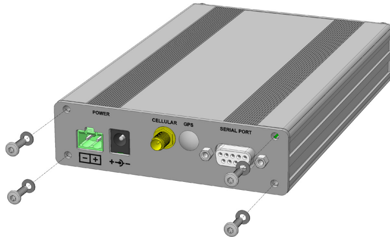
Figure 8 End Panel Screw Removal
