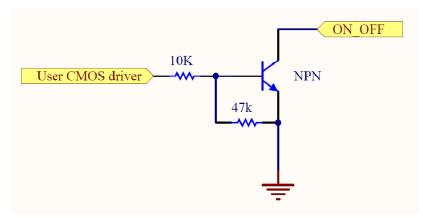
Figure 6 On / Off Pin Diagram
