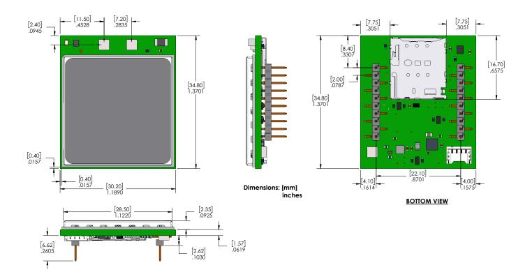
Figure 7 LTE910XFX Mechanical Dimensions
