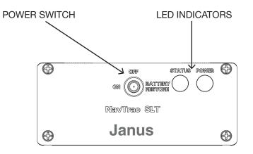
Figure 3 Front Controls and Indicators
