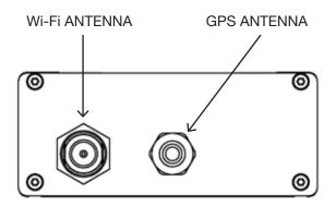
Figure 4 Rear Connections
