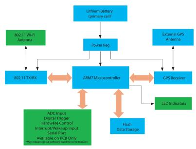
Figure 1 Wi-Fi Terminus NT-220LT Block Diagram
