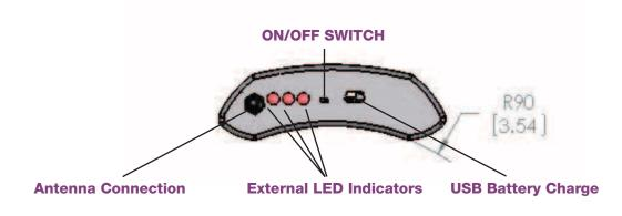
Figure 3 External Connections
