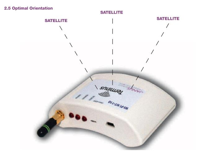
Figure 4 Wi-Fi Terminus NT-110ST Optimal Position
