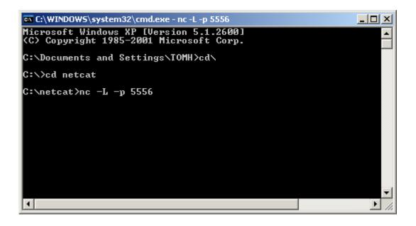
Note: The Server Computer must be connected to the Internet and able to except TCP/IP socket connections to the PORT defined in the TerminusGPS.py script. Please make sure the firewall is configured to allow this type of network traffic. If behind a wireless router you will need to specify routes to the Server Computer. Please call your IT professional to make sure your computer and network has the correct configuration for this. Janus cannot help you with your network settings.
