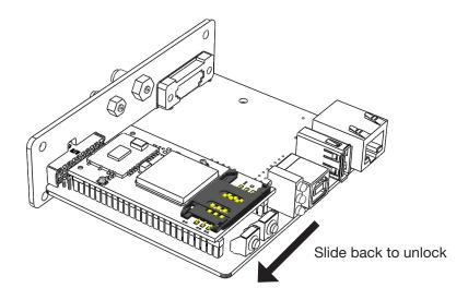
Step 3. Locate the SIM Card slot on top of the Terminus Plug-In board.
