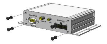
located on the back panel of the 400AP where the DB9 and lock header are located.
