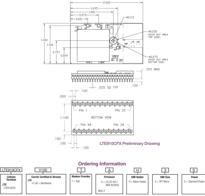
Example: Part Number – LTE910CFXV100TAH3S = LTE Cellular Cellular Modem Worldwide, Certified; Telit Modem; Standard Firmware with a U.FL Connector with a Variable Voltage with no configuration options.
