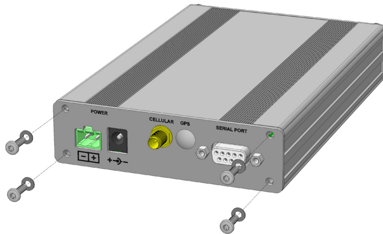
Figure 10 End Panel Screw Removal
