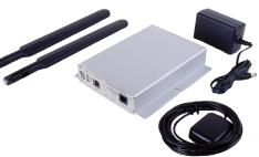
Integrating Telit's LE910C1-NF LTE module as their cellular engine, the LTE910PS POTSwap units operate in LTE bands 2, 4, 5, 12, 13, 14, 66, 71 with fallback to HSPA+ bands 2, 4, and 5. North American carriers include: Verizon and AT&T. Rogers, Bell and Telus versions will be available soon for Canadian customers.
