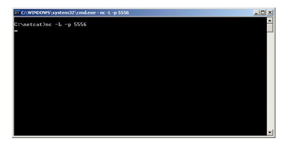
Note: The Server Computer must be connected to the Internet and able to accept TCP/IP socket connections to the PORT defined in the TerminusS2G.py script. Please make sure the firewall is configured to allow this type of network traffic. If behind a wireless router you will need to specify routes to the Server Computer. Please call your IT professional to make sure your computer and network has the correct configuration for this. Janus cannot help you with your network settings.
