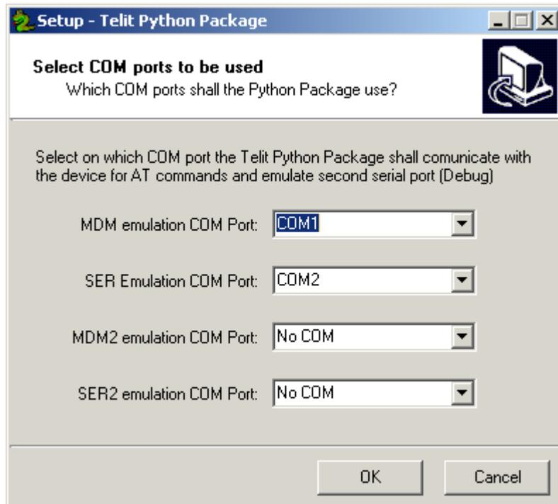
MDM emulation COM Port: This is the only port that must be assigned. The MDM assignment is used for the following tasks:
